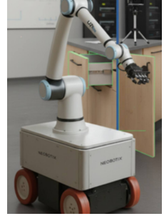
Figure 1: Steve coordinates its mobile base, arm, and PSYONIC hand while interacting with articulated furniture. Door traversal adds doorway and door-sweep constraints.
