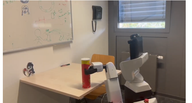
Figure 2: The existing HSR setup provides navigation and manipulation; this project adds metric-semantic mapping, task execution, and VLA manipulation.
