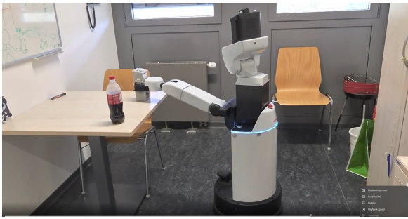
Figure 2: The existing HSR setup provides navigation and manipulation; this project adds metric-semantic mapping, task execution, and VLA manipulation.
