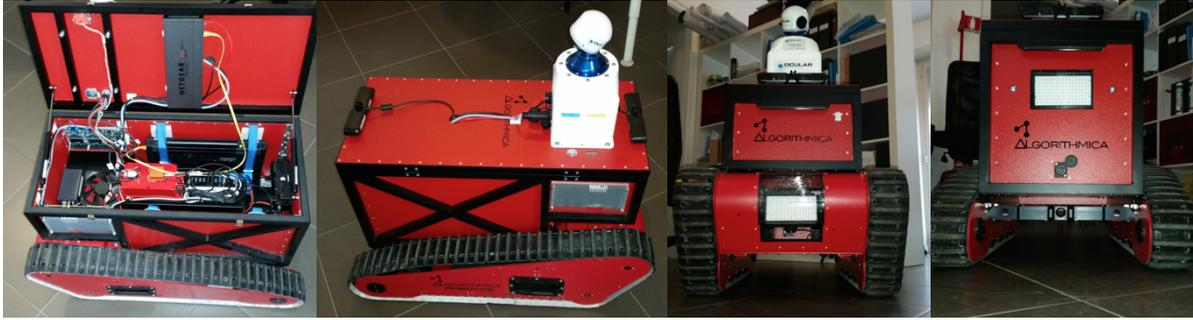
Figure 1 – The designed and constructed ROVINA robot (here depicted without the camera array).
