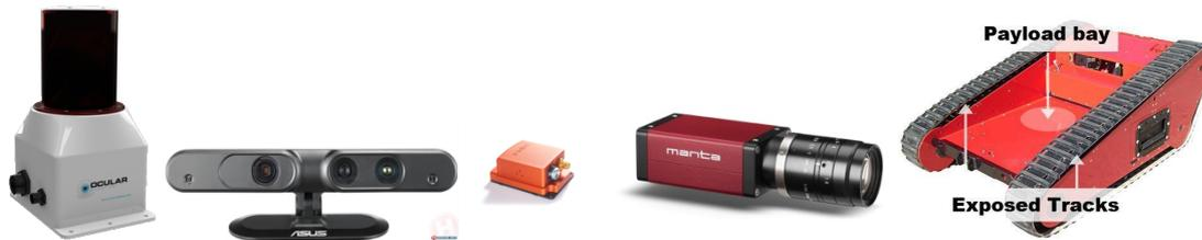
Figure 2 – A subset of the sensors and the base of the ROVINA robot platform.
