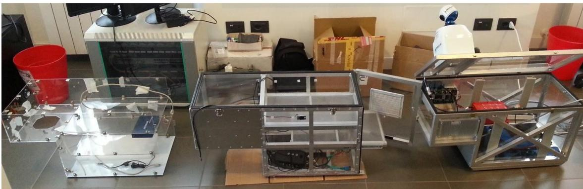
Figure 4 – Three iterations of the robot chassis design process.
