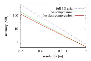
Fig. 10. Left: Evolution of the memory usage while mapping the FR-079 corridor dataset (resolution 0.05 m). Right: Effect of resolution on memory usage of the Freiburg outdoor dataset. Note that a logarithmic scaling is used.
