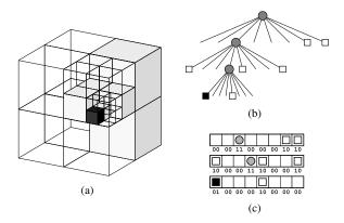
Fig. 2. Example of an octree storing free (shaded white) and occupied (black) cells (a), the corresponding tree representation (b), and the corresponding bitstream for compact storage in a file (c). The complete octree structure can be stored using only six bytes, 2 bits per child of a node.
