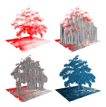
Fig. 1. 3D representation of a tree as a point cloud (top left), elevation map (top right), multi-level surface map (bottom left), and using our approach (bottom right).
