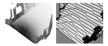
Fig. 4. A single 3D scan of the corridor dataset recorded with a tilting scanner (left) is converted to a maximum-likelihood map (right). Free cells are shown in white, occupied cells in black.
