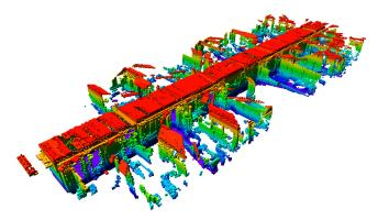
Fig. 8. 3D map of the corridor of building 079 on the Freiburg campus, as seen from the top. The structure of the adjacent rooms has been partially observed through the glass doors (size of the scene:  $43.8 \,\mathrm{m} \times 18.2 \,\mathrm{m} \times 3.3 \,\mathrm{m}$ ).
