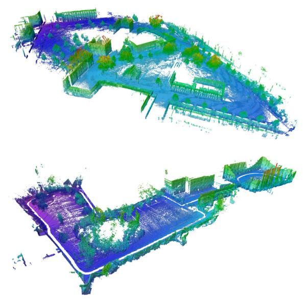
Fig. 9. Resulting octree maps of two outdoor environments at  $0.2\,\mathrm{m}$  resolution. For clarity, only occupied volumes are shown with height visualized by a color (gray scale) coding. Top: Freiburg campus (size of the scene:  $292\,\mathrm{m} \times 167\,\mathrm{m} \times 28\,\mathrm{m}$ ), bottom: New College (size of the scene:  $250\,\mathrm{m} \times 161\,\mathrm{m} \times 33\,\mathrm{m}$ ).
