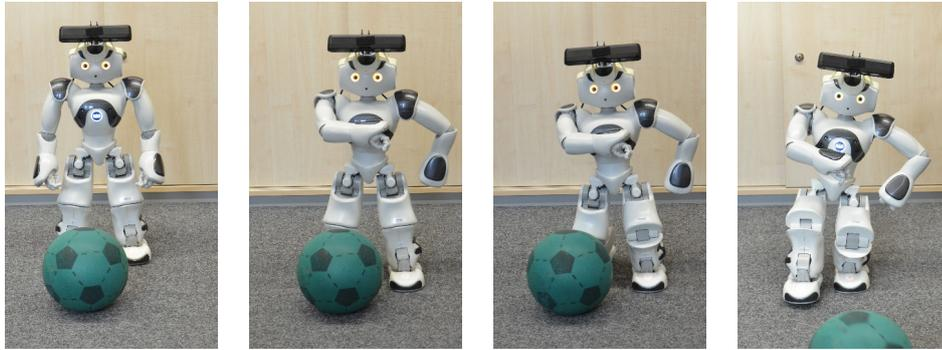
Fig. 8. Pushing: In our implementation, the push action includes tracking the ball locally, positioning relative to the object, and kicking it in the forward direction.
