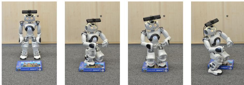
Fig. 9. Stepping onto: The step onto action includes stepping onto the object and also stepping down according to a footstep plan.
