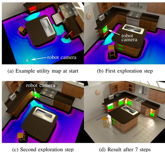
Fig. 5. Progress of exploring a kitchen scene. The robot first estimates utility maps for multiple articulation configurations. The robot then chooses the articulation object and view point with the highest utility (b). Afterwards, the algorithm computes utility maps from the new location taking into account already observed regions. Regions of interest are marked in red, observed regions in green, and the robot’s camera is symbolized as a white pyramid.
