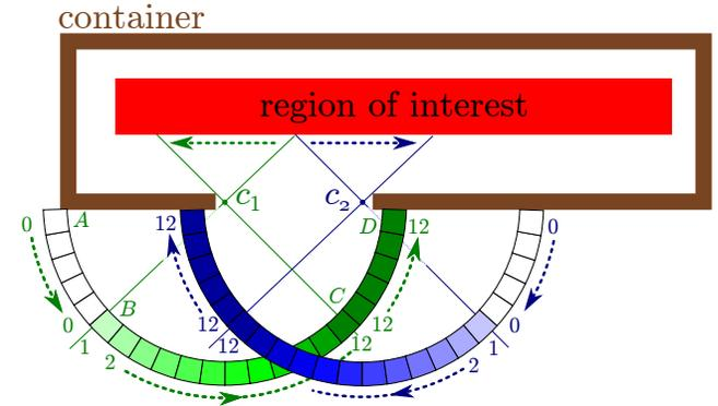
Fig. 3. Estimating the information gain map by calculating the integral images of two spherical cameras  $c_1$  and  $c_2$ . The numbers indicate the estimated information gain accumulated by pivoting rays through the camera center in the direction indicated by arrows.
