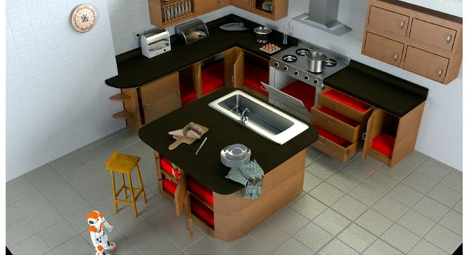
Fig. 1. Nao inspecting a kitchen environment. The robot’s task is to search for an object in the user-defined regions of interest marked in red. Kitchen model based on [1].
