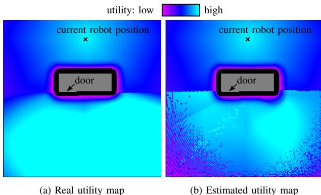
Fig. 4. Comparison of the real utility map obtained by exhaustive sampling and the estimated utility map generated by Alg. 6 for the scene with a cupboard shown in Fig. 2.
