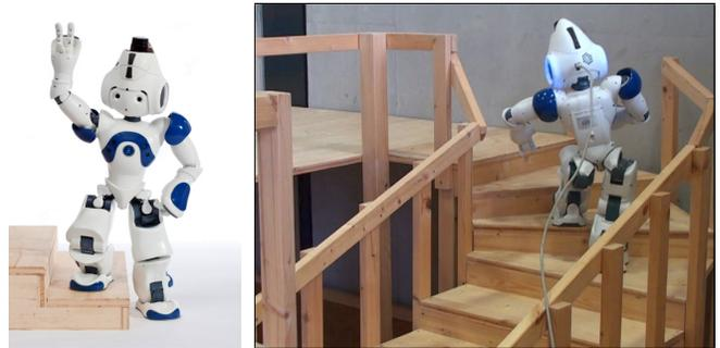
Fig. 1. *Left*: Our Nao humanoid is equipped with two low-cost monocular cameras and a Hokuyo 2D laser scanner on top of the head (photo: B. Schilling). We use 2D laser range data for globally localizing the robot and images of the lower camera (located below the eyes) for detecting edges corresponding to stairs. *Right*: Nao climbing up a spiral staircase using vision and laser data.
