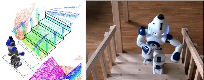
Fig. 1. *Left:* Model of the staircase reconstructed from a 3D point cloud acquired with a laser-equipped Nao humanoid. *Right:* The robot is able to climb the staircase based on the learned model of the environment.
