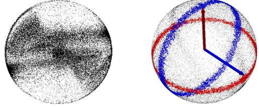
Fig. 6. The normalized difference vectors  $V$  from the point cloud in Fig. 3 as points on the unit sphere (black dots). *Left*: With uniform sampling, there are no distinct main directions. *Right*: Using improved sampling considering neighboring information, the distinct rings corresponding to the main directions can be clearly identified (indicated by their normal vectors as red and blue arrows).
