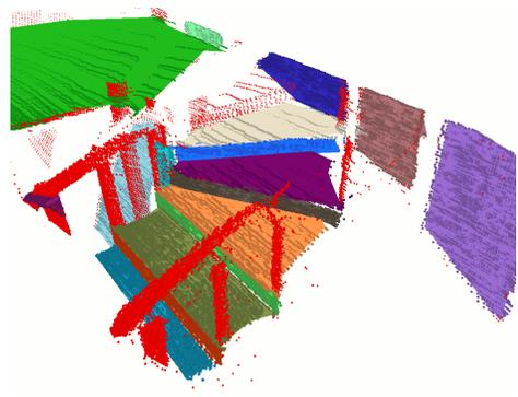
Fig. 8. Segmentation using scan-line grouping on another dataset of the upper part of our spiral staircase. Several steps are extracted successfully including their vertical faces. The large green area corresponds to the upper level whereas segments on the right refer to a distant wall.
