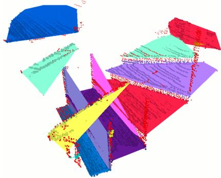
Fig. 10. Segmentation of our improved two-point algorithm on the dataset of the upper staircase. The same steps as in scan-line grouping are segmented reliably. Even though some vertical faces are missing, the extraction result can be used for reconstructing the staircase model.
