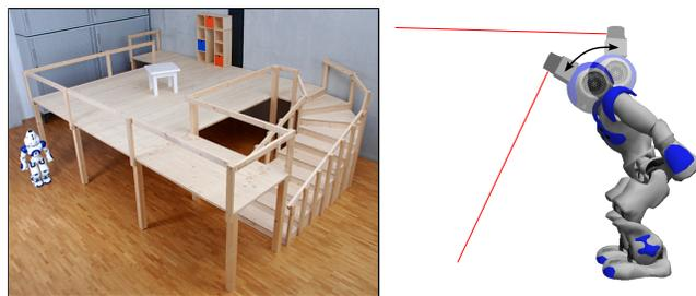
Fig. 2. *Left:* The two-level environment in which the robot is navigating. *Right:* The Nao humanoid is acquiring a 3D point cloud of the environment by tilting its head with the 2D laser range finder on top.
