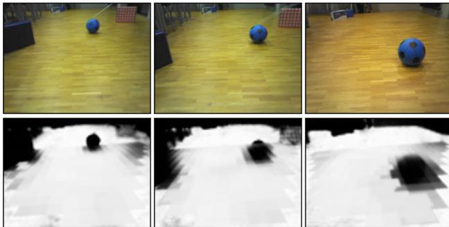
Fig. 7. We achieve reliable traversability estimates also in presence of moving obstacles. We rolled a soccer ball multiple times in front of the robot's field of view while navigating. The top row shows the camera images and the bottom row the corresponding traversability estimates.
