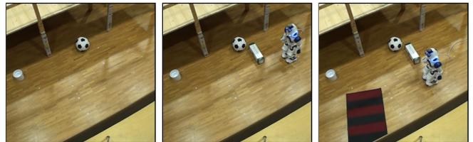
Fig. 7. Left: scene during training (robot outside the cameras field of view). Middle: new but similar-looking objects do not trigger re-training. Right: Adding the carpet is interpreted as a substantial change and re-training is triggered.
