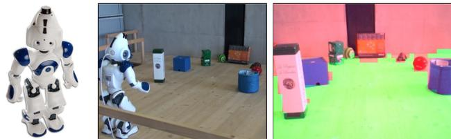
Fig. 1. Left: Humanoid robot Nao equipped with a Hokuyo laser scanner in its head. Middle: Navigating robot. Right: Corresponding image taken by the robot’s onboard camera together with traversability labels estimated by our approach (green refers to traversable, red to non-traversable areas). This image is best viewed in color.
