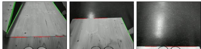
Fig. 2. By extracting lines from the camera images, the robot can detect the start (left) and end (center and right image) of the ramp. The detected horizontal lines are marked in red.
