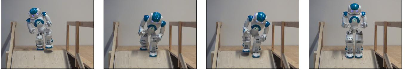
Fig. 3. Nao executes a single step onto the ramp after detecting the start in its camera image.
