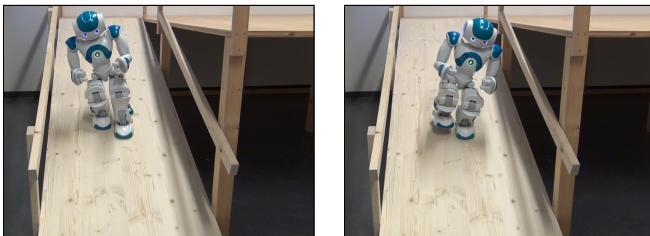
Fig. 4. Nao executes statically stable steps on the ramp and regularly corrects its heading based on IMU data.
