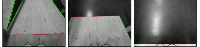
Fig. 2. By extracting lines from the camera images, the robot can detect the start (left) and end of the ramp (center and right image). The detected horizontal lines are marked in red.
