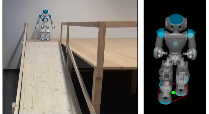
Fig. 1. *Left:* The Nao humanoid in a two-level environment, connected by a ramp. *Right:* Support polygon (red) and projected center of mass (green dot) for a double-support phase on the ramp.
