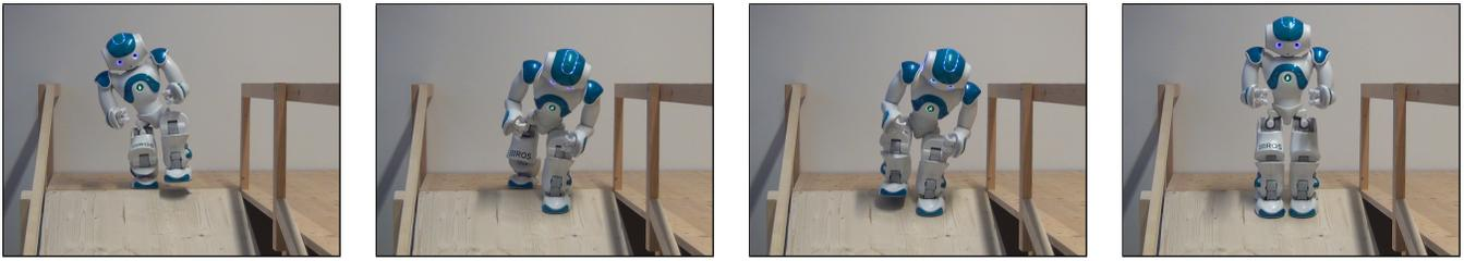
Fig. 3. Nao executes a single step onto the ramp after detecting the start in its camera image.
