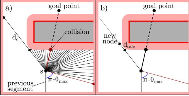
Fig. 4: Creation of a new node. Left: If a collision along the direct line from the robot’s pose  $s$  to the goal point is detected the framework systematically searches for possible free rotations. Right: If a free rotation is found, a new node is created and the path search continues using the new node.
