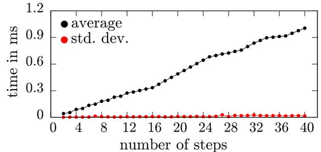
Fig. 9: Run times for footstep step calculation. We used five different sufficiently long paths and averaged over 5000 iterations per step count.
