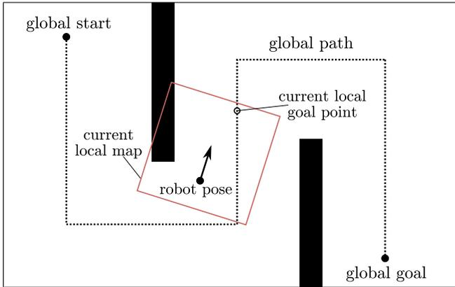
Fig. 3: Global path following. In order to follow a global path, the framework selects local goal points using the furthest reachable point of the global path that lies within the local map.
