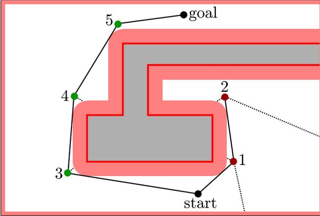
Fig. 5: Example search graph. The search first inspected the nodes 1 and 2 but did not find a free way to the goal and thus continued starting from node 3. The order of processed nodes during the search is thus: start-1-2-1-start-3-4-5-goal.
