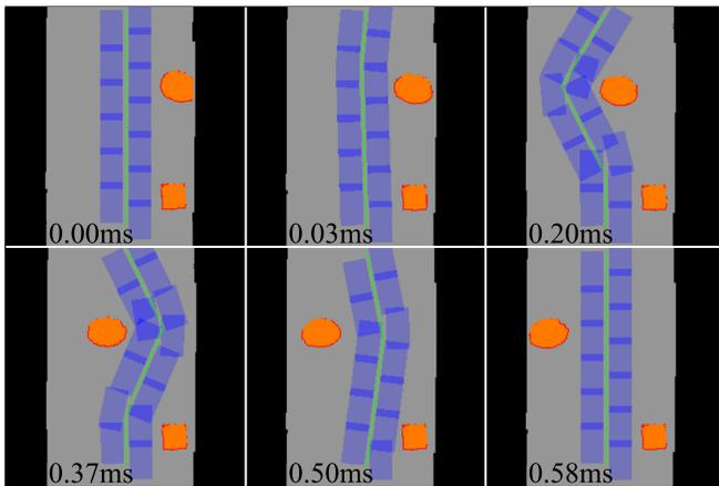
Fig. 11: Ball rolling in front of the robot. When a ball is rolled in the path of the robot, our framework allows a reaction in real time.
