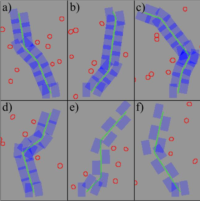
Fig. 7: Example 2D paths with footsteps calculated by our approach. We sampled a random numbers of objects in the local map. Images a-d show plans for the step distances for the Nao robot. In Figs. e and f we have increased the step distances to show resulting paths for a robot with a larger step length. All images are cropped to the regions that contain the corresponding 2D path.
