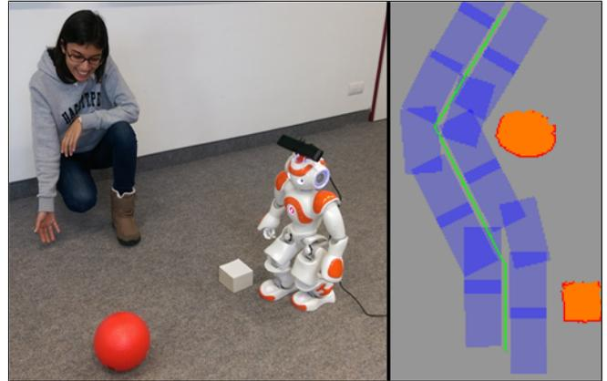
Fig. 1: Real-time footstep planning. Our framework is capable of adapting to local changes in the environment at a delay of just 18 ms on average.
