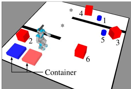
Fig. 7. Nao humanoid in a simulated environment. The clean up task is complete when the robot has placed all of the six objects into their corresponding container (Scenario 1). Optional movable obstacle locations are marked with a \* and are used in Scenario 2.
