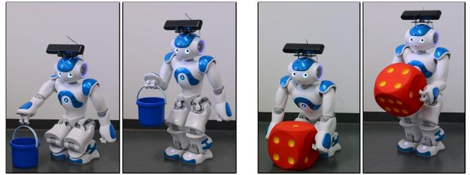
Fig. 3. Whole-body motion for picking up a bucket by grasping its handle (left) and for picking up a cube with both arms (right).
