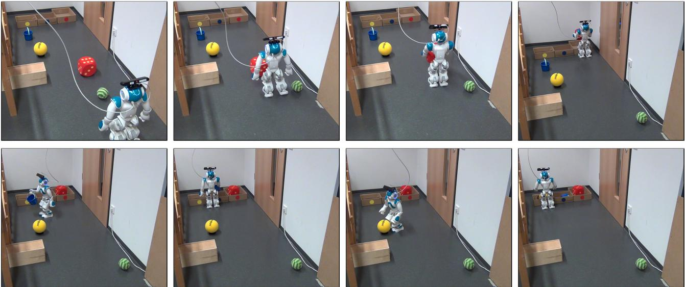
Fig. 8. A Nao humanoid cleans up a cluttered environment using our approach. The robot first has to move the small ball aside, and then pick up the red cube. After placing it into a container, the robot can clean up the remainder of the scene. A video of this sequence accompanies the paper submission.
