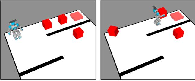
Fig. 4. A clean-up scenario in which the red cubes have to be transported into the container at the top right. The object configuration does not allow the robot to clean up one object after another (left). Instead, it has to move a blocking cube out of the way first (right). The symbolic planner samples and grounds intermediate locations such as the one in the corner as needed.
