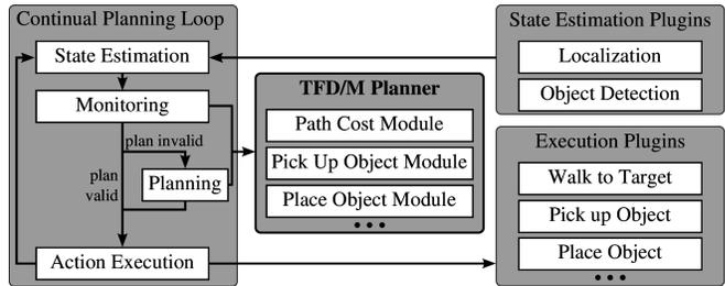
Fig. 2. Overview of the TFD/M planner in the continual planning loop with its modules and plugins.
