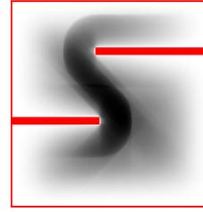
Fig. 5. Object placement costs from motion planning between sampled start and end points in the environment of Fig. 4 (darker: higher costs).
