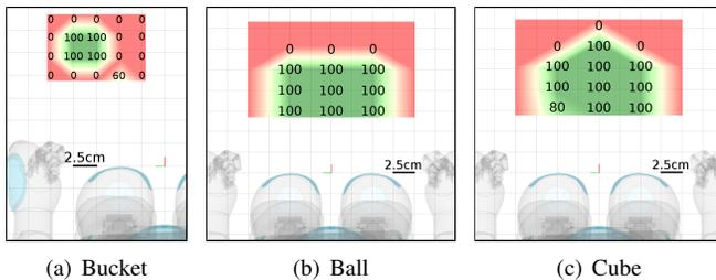
Fig. 6. Success rate for picking up a bucket, a ball, and a cube at different positions relative to the robot ( $N=5$  tries for each location). The numbers indicate the success rate of the object placed at the corresponding location while the robot remains at the same location, as seen from the top.
