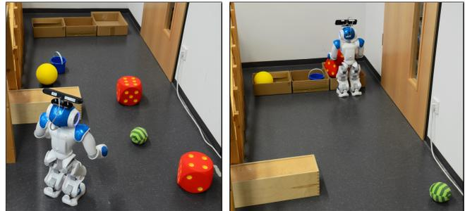
Fig. 1. Left: Example tidy-up task to be solved by our integrated system. All larger objects have to be picked up and placed into their corresponding container. To complete this task, the robot has to reason about a sequence of actions such as picking up an object, walking to a target location, and moving an object out of the way. Right: The final state with all objects tidied up, except for the green ball that was considered as clutter and moved aside by the robot with its foot.
