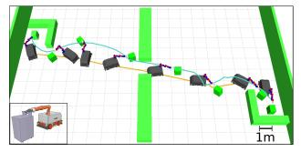
Fig. 1: Configuration sequence of a solution path generated by our BI<sup>2</sup>RRT\* planning framework for the complex task of maneuvering a cart out of a parking lot and into another. The orange and blue line represent the corresponding trajectory of the mobile base and end-effector.
