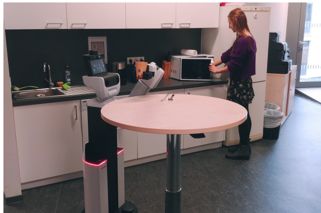
Fig. 1: Motivation of our approach. While the user moves to a microwave, the robot predicts it can offer service at the table by providing a cup.
