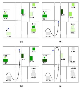
Fig. 5: Evolution of the belief over time for an example human trajectory. As can be seen, the initial belief based on the interaction model (a) is continuously updated with new observations (b), (c), (d). Possible goals are shown in green with their probabilities to be the navigation goal: the darker the green the higher the probability. Doors are colored in grey and walls in black. The human is depicted as blue dot with their trajectory as dashed line.
