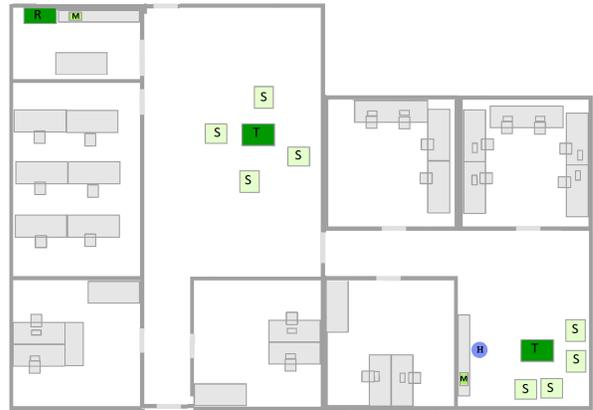
Fig. 2: Example for the goal prediction based *solely* on the interaction model after a detected worktop interaction. Objects are color coded with respect to their likelihood to be the next movement goal of the human (H). The darker the green the higher the likelihood. Object names are abbreviated: dining table (T), microwave (M), refrigerator (R), and sofa (S).
