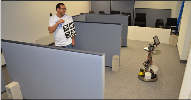
Fig. 6. The robot and the user with a board of ArUco markers to simplify pose estimation in the real-world experiment.
