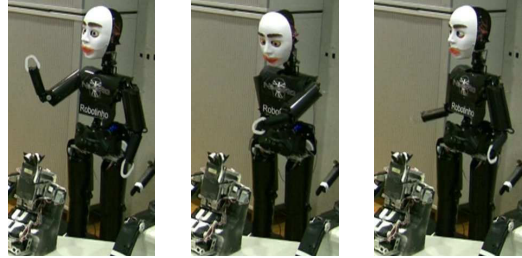
Fig. 1. Our humanoid robot interacts with people using multiple modalities such as speech, facial expressions, eye-gaze, and gestures.
