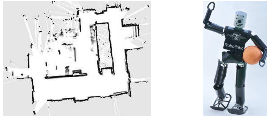
Fig. 1. A learned map by our approach using noisy and short-range laser data acquired with the humanoid Robotinho.
