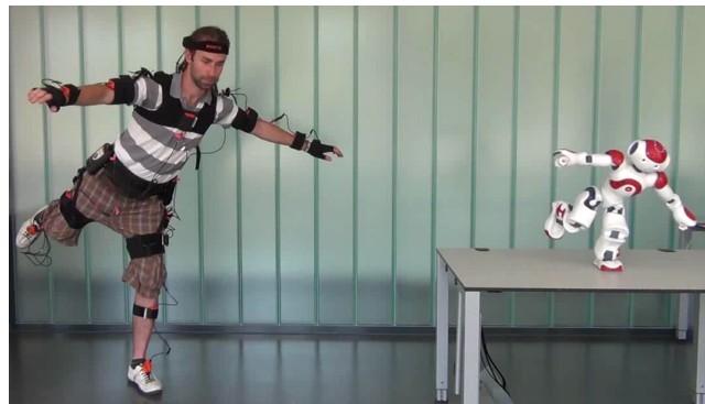
Figure 1: Nao imitating complex whole-body motions. The robot actively balances its center of mass to achieve static stability.
