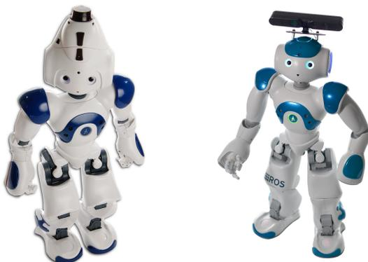
Fig. 5. Nao humanoids used for the evaluation of our work, using a head-mounted 2D laser range finder (left) and an RGBD-camera (right).
