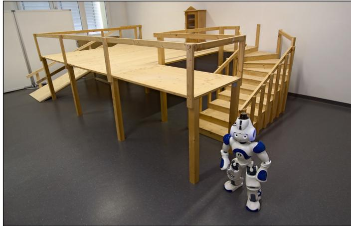
Fig. 1. Nao humanoid with a laser range finder navigating in a complex environment containing multiple levels, a staircase, and a ramp (Environment I). Using our localization approach, the robot is able to accurately estimate its 6D pose while walking and climbing stairs.
