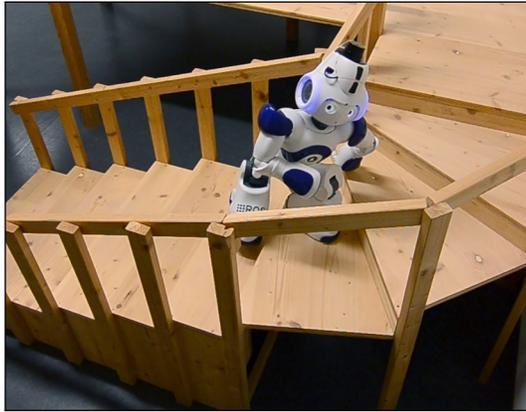
Fig. 11. Nao humanoid climbing a spiral staircase using our approach of combining vision and laser range data for localization to correct for motion noise.
