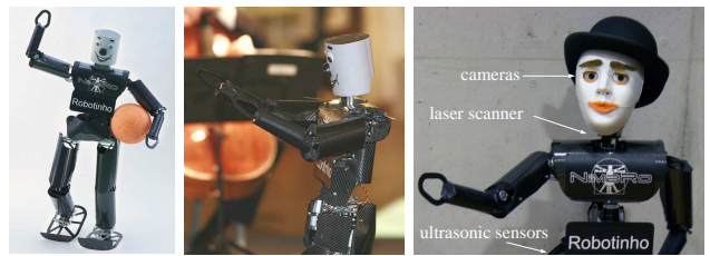
Fig. 2. Our robot Robotinho was initially used as soccer player in the RoboCup Humanoid League. He conducted The 12 Cellists of the Berlin Philharmonic in September, 2006. The right image shows the communication head as well as the position of the cameras and distance sensors.
