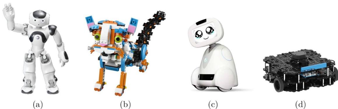
Figure 1: Examples of different robot design classes: (a) an anthropomorphic NAO robot [26], (b) a zoomorphic LEGO BOOST robot [27], (c) a caricatured Buddy robot [28], (d) a functional Turtlebot Waffle robot [29].
