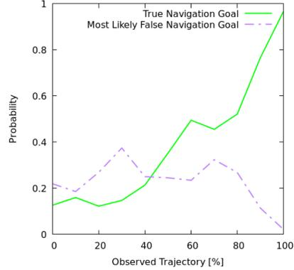
(b) Evolution of the belief about the navigation goal with respect to the percentage of the observed length of a typical trajectory, which is depicted on the left.
