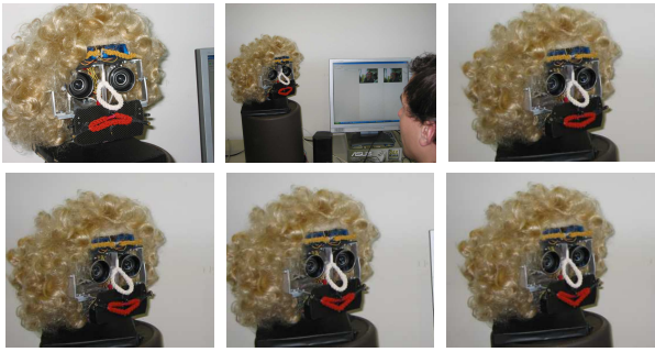
Figure 8: This figure shows continuous changes of the facial expression. Initially, the robot is in a mood corresponding to a blending of sadness and fear since it is alone (top left image). Then, the robots suddenly detects a person and changes its facial expression towards surprise (center image in the first row). Afterwards, the robot gets happy because the person starts to interact with it (following images).
