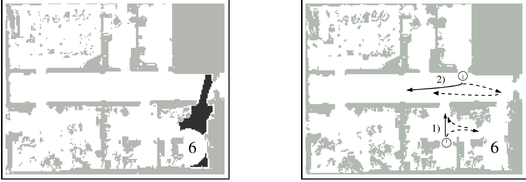
Figure 2. The left image shows the visibility area for resting place 6. The right image shows for two scenarios the detours to the viewpoints to which the robot moves. The solid lines indicate the direct paths to the target locations of the robot and the dashed lines are the detours to the viewpoints.
